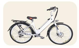
The Vee comes with a 36V 10ah battery. The top speed can reach 35km/h with a range of 40-50kms on electric only. With pedal assist, the range will increase to 60kms. Because the upper frame bar is removed, it allows the female gender to climb aboard more comfortably, creating the modern look of city bikes.
