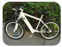
This ebike comes with a 48V 10ah battery. The top speed can reach 45 km/h with a range of 40-50 kms on electric only. With pedal assist, the range will increase to 60 kms. This is the perfect city bike and a good performer off-road. The Zoom comes with a 500 W motor. Weighs 25 kg
