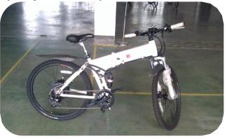
This ebike comes with a 36V 9ah battery. The top speed is 35km/h with a range of 30-35kms on electric mode only, on a 500W motor. With pedal assist, the range increases to 50-55kms.
